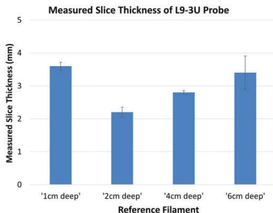
**Figure 4.** Results of the test for one probe. The bars showing the measured slice thickness at the given depths, the error bars are the standard deviation of the measurements obtained by performing the test across three regions of the probe face.
