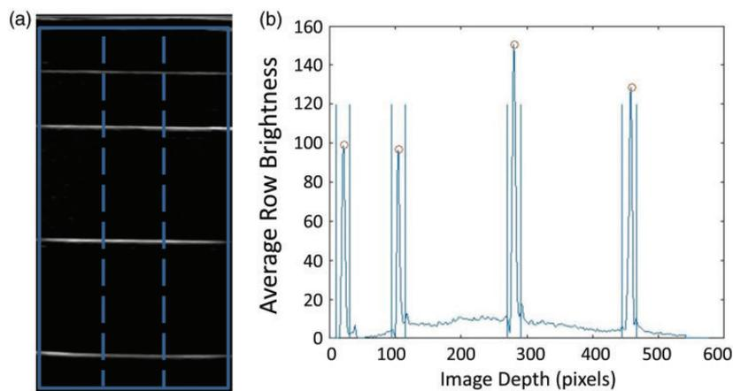
**Figure 2.** (a) Example composite image obtained at one probe position. The dotted line overlay showing the separation of the method into three regions of the probe face for an extension to the test. (b) Example 1D profile obtained by averaging the pixel values in each row of (a). Each detected peak corresponds to a visible wire in the phantom for this probe position.
