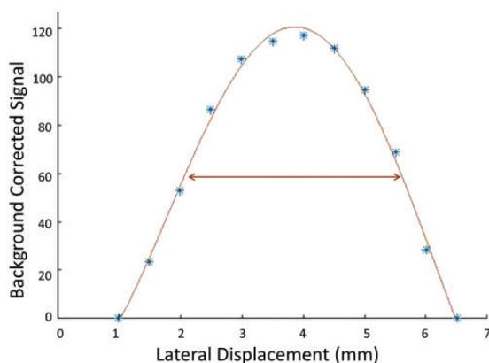
**Figure 3.** Example probe slice profile obtained using the described method. Asterisks show the background corrected signal obtained for one wire in the phantom across all composite images for the tested probe. The full width half maximum (FWHM) of the curve fitted through the data points was defined as the slice thickness at this wire depth for the probe.
