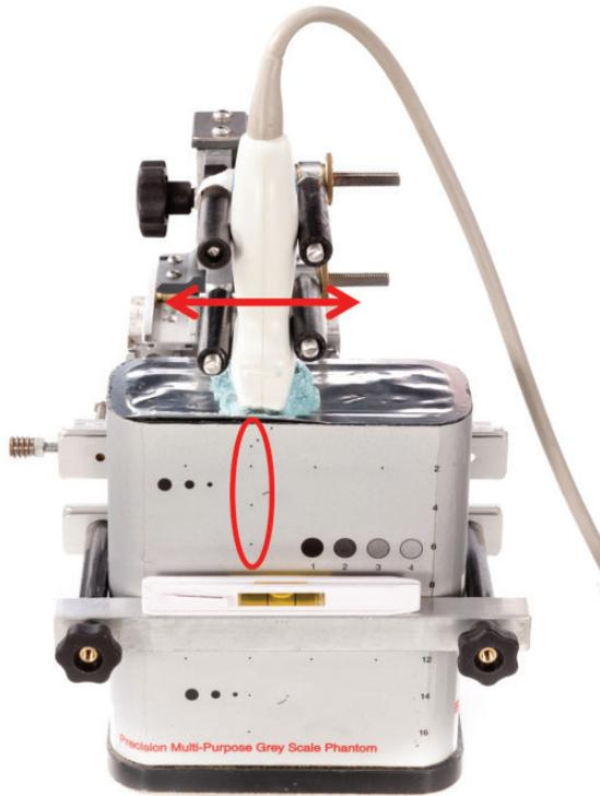
**Figure 1.** Phantom, jig and probe setup. The double headed arrow shows the direction of probe movement. The ring shows the wires in the phantom used in the test.
