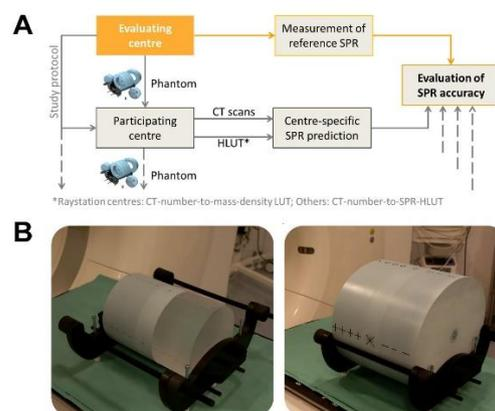
Figure 1: (A) Scheme of the study design. SPR: Stopping power ratio; HLUT: Hounsfield look-up table. (B) Experimental setup of the head (left) and body phantom (right) with the tissue surrogate inserts placed in the centre part of each phantom.
