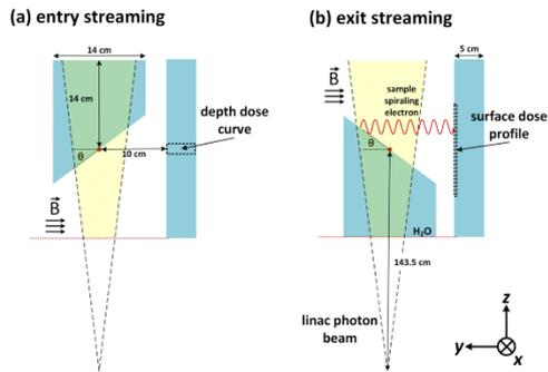
Figure 1: Schematic of EGSnrc simulation set-up of the (a) entry and (b) exit inclined phantoms.
