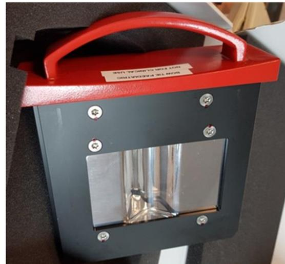
Fig 1: The paediatric bowtie filter. The thick central part of the filter reduced exposure fivefold.
